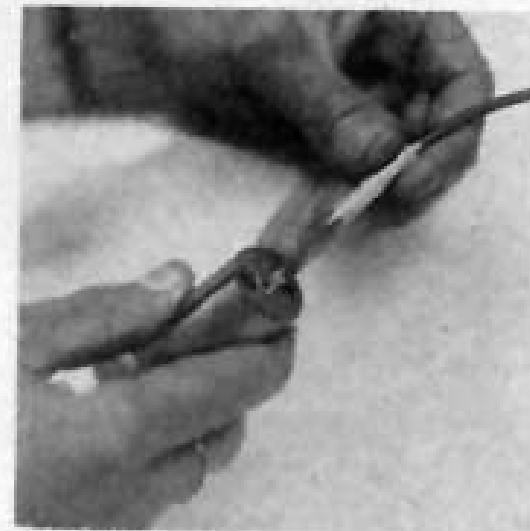
FIG. 54. SHOWING HOW TO REMOVE THE TAPER NEEDLE FROM THE THROTTLE OF THE TWO-LEVER CARBURETTOR
